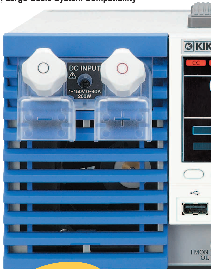
Detachable input terminals for ease of use.
